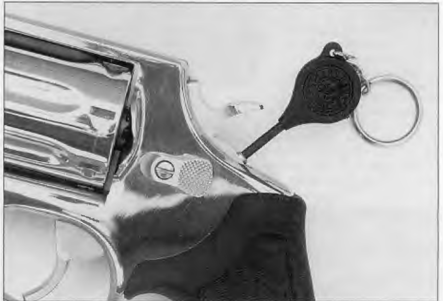
Taurus M617 .357 Magnum snubnose, right-side view. Note high-polish stainless steel finish, black neoprene-type grips and serrated ramp-type front sight. (right) Taurus key-lock safety system raises a pin and its shroud to impinge against the frame if someone attempts to roll the hammer rearward.
